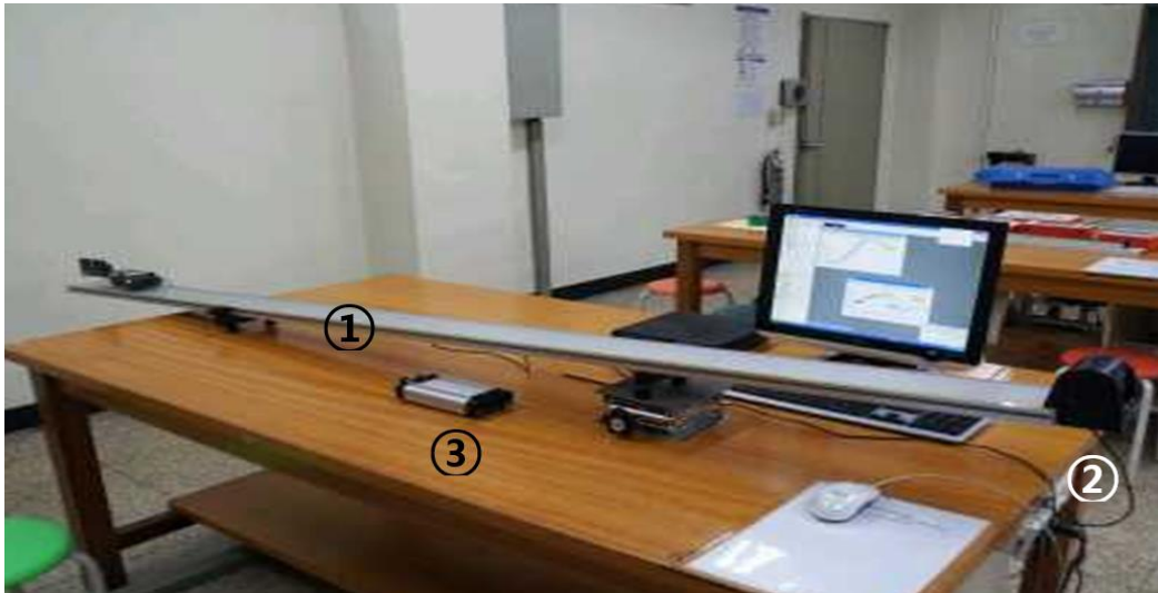
Fig. 1 Experimental setup. ① aluminum dynamic track system(ME-9779, PASCO), ② motion sensor(PS-2103A, PASCO), ③ cart
